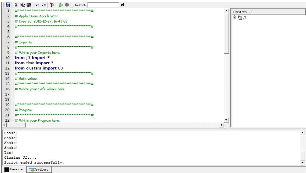
Figure 6. JFT program for a Freescale MMA7660FCT I2C based vibration test.
